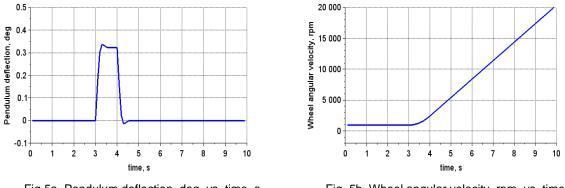
Fig 5a. Pendulum deflection, deg, vs. time, s
