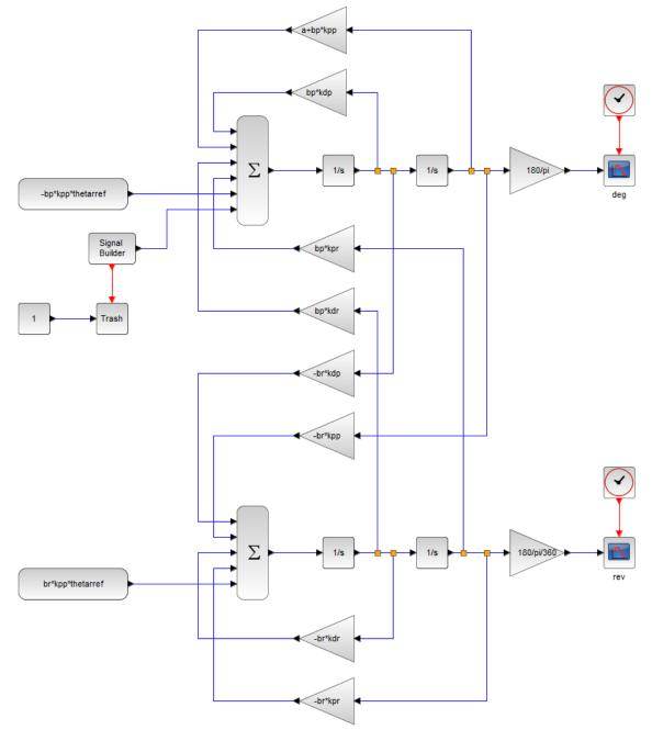
Fig. 4. Subsystem for working out a solution to system ODEs (8) (wheel angle)
